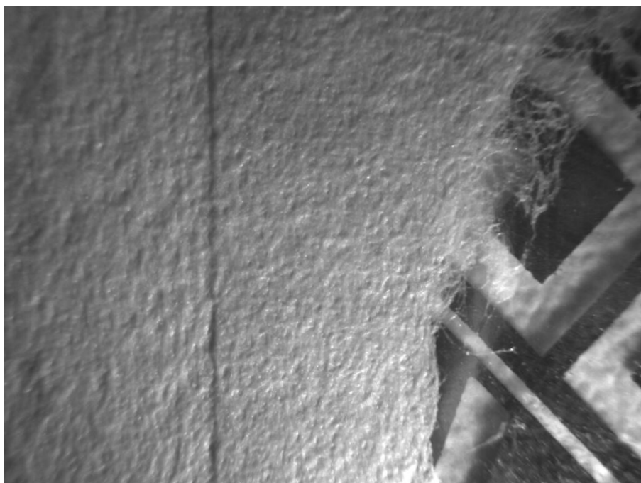
Spectral luminescent magnifier Regula 4177: Infrared oblique light (880 nm) 1x
