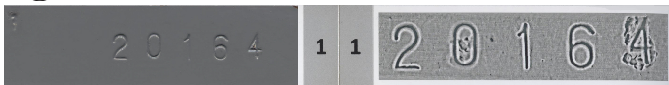
Press processing (calking)
