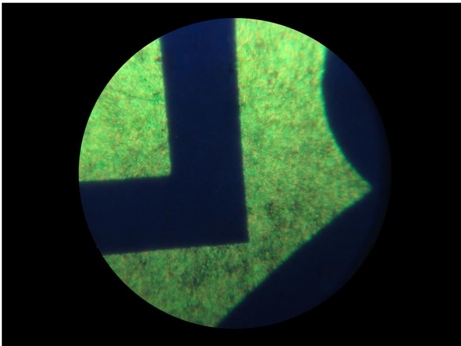
Examination in ultraviolet spectral range – 254 nm
