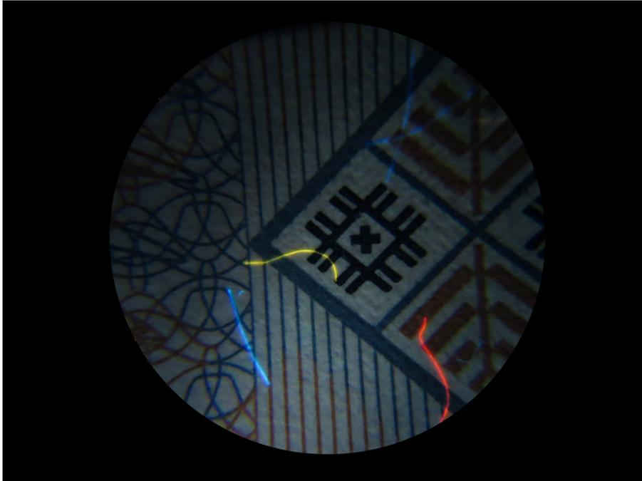
Examination in ultraviolet spectral range - 400 nm
